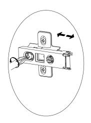
Move panel left and right to match with the screw shown.
