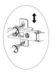
When the panels connected by the hinge cannot close properly, please loose the 4 screws and move the the panel top and down to relocate the position of hinge with the screws shown.
