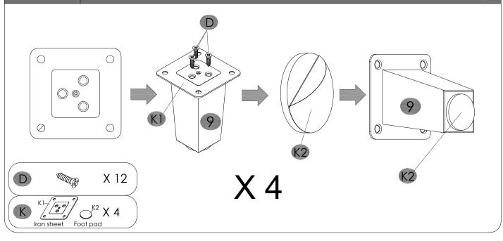
STEP 8 After the seventh step, fix the components(9) to the board(4) using screws(D).
