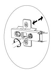
Move panel in and out to match with the screw shown, and retighten the 4 screws.
